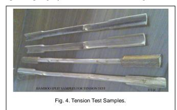
The portion between the grips was marked with a distance of one cm interval. Average area was calculated on three sections, two at ends and one at centre. Gauge length  $5.64 \times (A)1/2$  was marked and the extensioneter was fixed to record the elongation at loading intervals.
